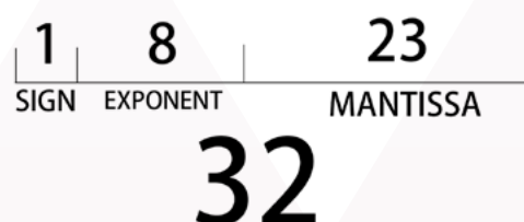
Figure1, the distribution of bits in a floating point number with single precision.
